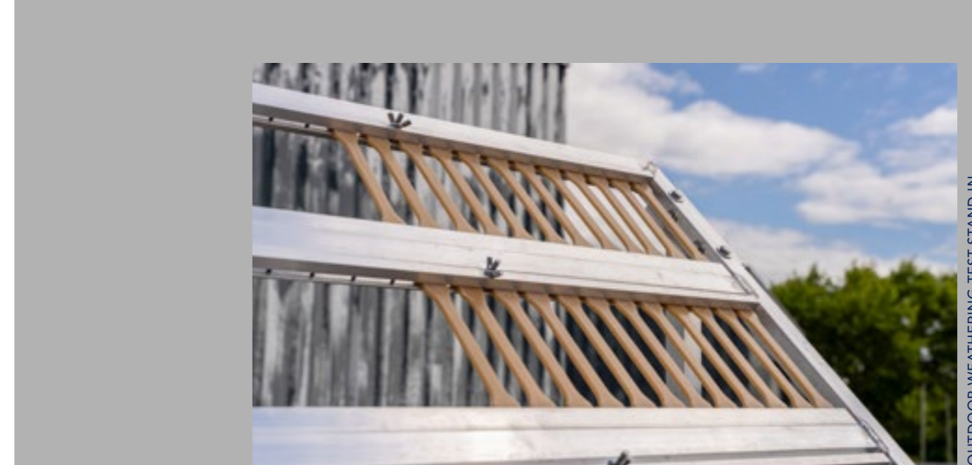
OUTDOOR WEATHERING TEST STAND IN THE BeBio2 RESEARCH NETWORK. Photo: IfW
