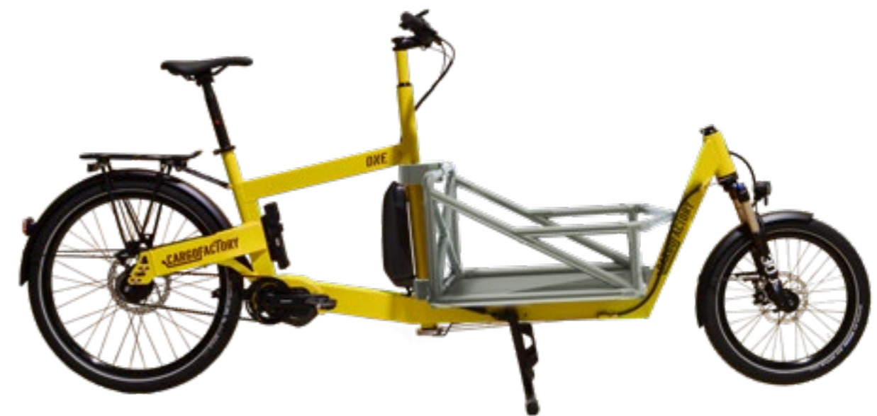
THE DEMONSTRATOR, AN INTEGRABLE BASKET FOR AN ELECTRIC CARGO BIKE, COMBINES ALL THE CENTRAL SCIENTIFIC KNOWLEDGE OF THE ALLEGRO PROJECT IN A COMPLEX PRODUCT (FIGURE 1). Photo: ALLEGRO/CargoFactory
